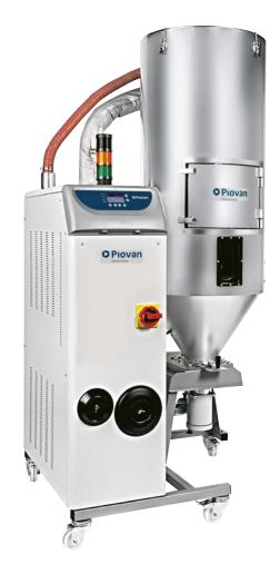
Double desiccant tower models, with an airflow rate from 50 to 150 m3/h, supply air at a dew point lower than -50°C. The process air temperature can be set up to 200°C (HT version). The DP 604 - DP 615 Dryer Series is
